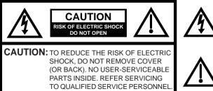
The lightning flash with arrowhead symbol, within an equilateral triangle is intended to alert the user to the presence of uninsulated dangerous voltage within the product's enclosure that may be of sufficient magnitude to constitute a risk of electric shock
